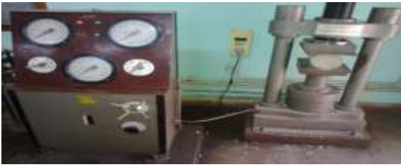
Figure 5.4 Split Tensile Test on Concrete Cylinder
