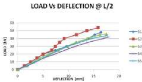
Figure 5.8 Load Vs Deflection Curve at L/2 for S1 to S5
